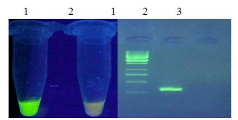
**Fig. 1(a).** LAMP optimization 1: Positive reaction 2: Negative reaction
